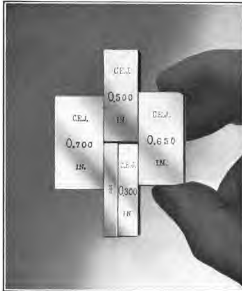
FIG. 199. — FIVE PIECES WRUNG TOGETHER
